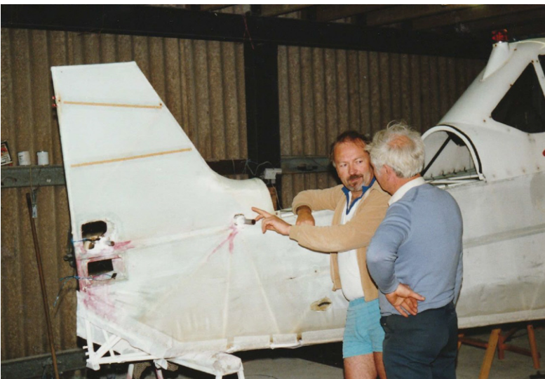
Dave Masterson (right) talking to Guy Applebeck, checking out G-TOWS ("This is where they crack"). Notice the red dye penetrant crack detection fluid.
