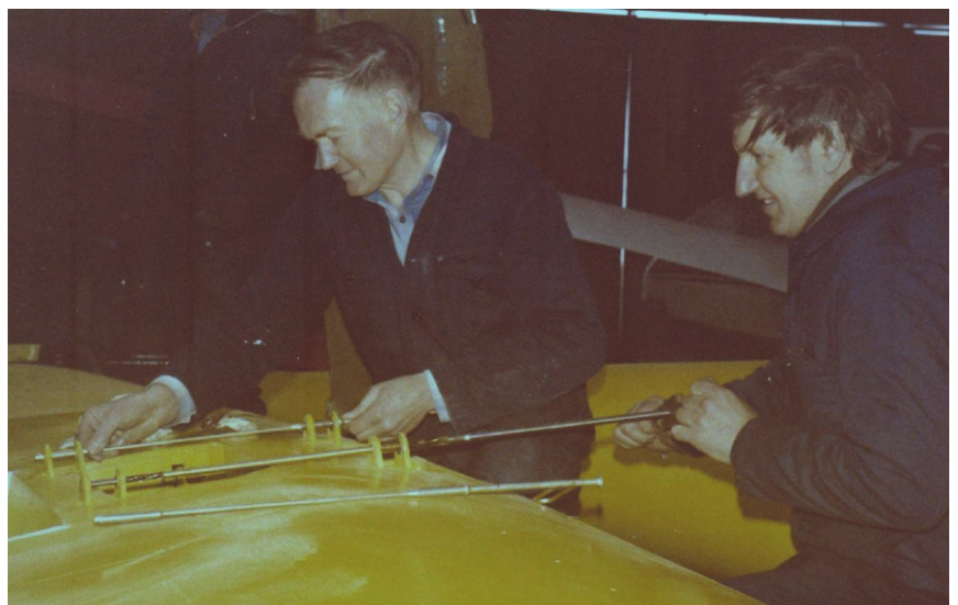
Engineering Genius – Ken Fixter (right) and Peter Philpot, reaming Rhubarb and Custard's wing for oversize main pins.
